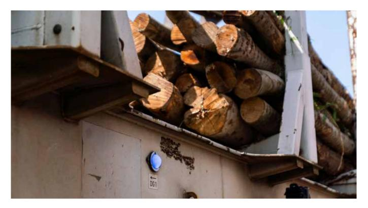
On-site visualition in real-time via signal lamps. Automatic load weight monitoring indicates in real time during loading: Overloading, asymmetric loading, wheelset and wheel disc overloading, inadmissable load distribution on the bogie, loading level and loading is ok.
